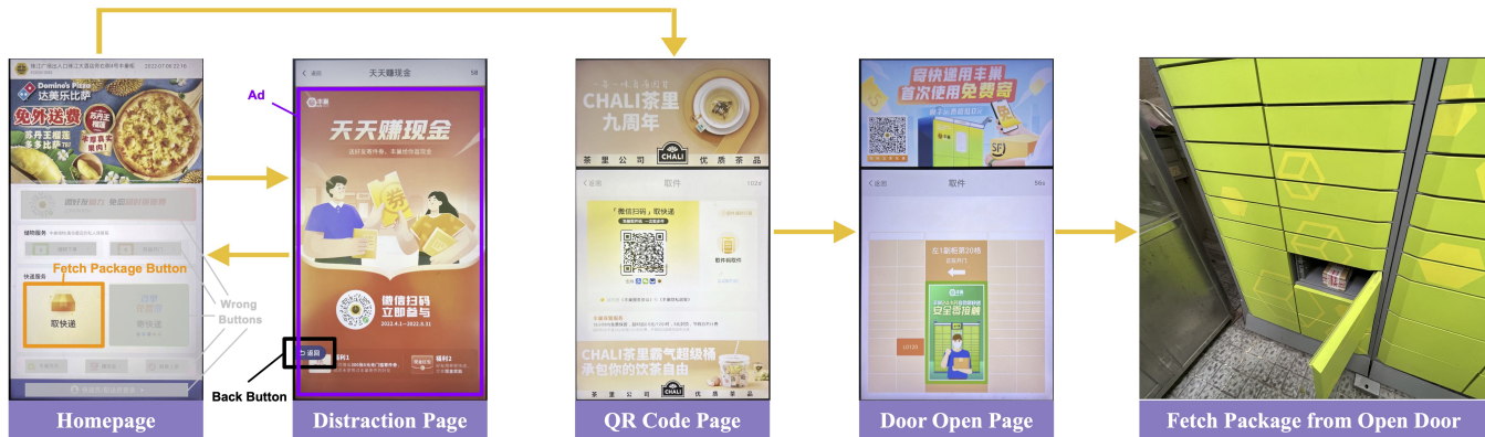
Figure 3: Task flow of the HiveBox parcel locker touchscreen. The user starts with the Homepage. To fetch a package from a HiveBox, the user needs to first tap the “Fetch Package” button on the homepage, which consequently reveals the QR Code Page. The user needs to scan the QR code to unlock the door. The QR code will not be revealed if the user clicks the wrong button, which instead reveals a Distraction Page (e.g. an advertisement and a back button), and the user needs to press the “back button” to return to the previous page. The compartment location is shown on the Door Open Page after the QR code is scanned for user authentication.
