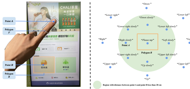
Figure 6: Illustration of Touchscreen Interaction with FetchAid. Left: Point A and Polygon F track the user’s fingertip, while Point B and Polygon R track the target button (e.g., “Fetch Package” button). Right: Voice feedback and guidance are provided for different directions based on the relative position between the fingertip (Point A) and the target button (Point B). When the distance between Point A and Point B is less than 20 cm, users are reminded to move slowly. Distances in this step are heuristically determined using perspective projection.
