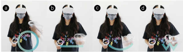
Figure 5: Four canvas invocation gestures of the motion canvas, and use the displacement of the handle directly as the input of the gesture action: a) circle action. b) straight action. c) curved action. d) fold action.
