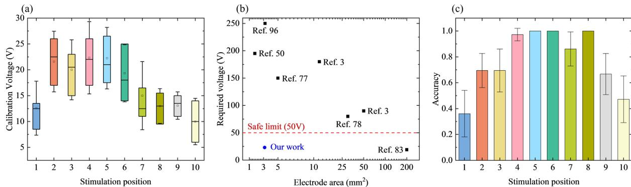
**Figure 4: Calibration and position recognition results. (a) Box plot displaying the calibration voltage results. (b) The comparison of the required voltage for this work and previous research. (c) Position recognition accuracy for different stimulation positions at a fixed stimulation time of 0.5s.**
