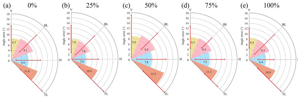
**Figure 6: The direction recognition results under the stimulation intervals of 0% (a), 25% (b), 50% (c), 75% (d), and 100% (e) of the stimulation time. (H: horizontal direction, V: vertical direction, BL: bottom-left top-right direction, TL: top-left bottom-right direction) The radius of the colored sector represents the angle error. The smaller the radius, the lower the angle error, and the interval of 25% of stimulation time led to the lowest error in these directions.**
