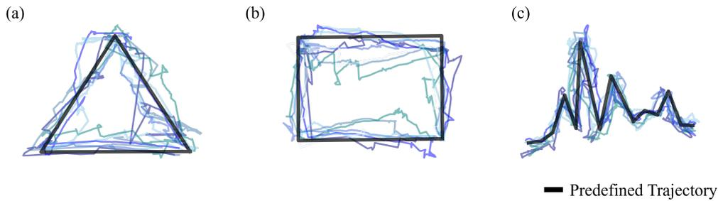
**Figure 9: The trajectories of the two training tasks (TN1, TN2) and T1. The blue lines were the participants' finger-moving trajectories, while the black lines were the predefined trajectories: a) TN1 (follow triangle guidance); b) TN2 (follow rectangle guidance); c) T1 (find line chart's trend)**
