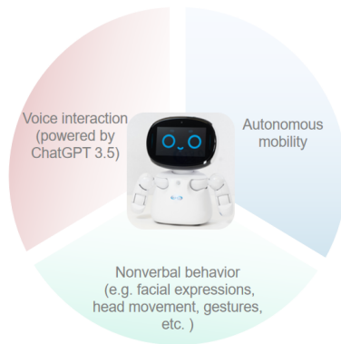
Fig. 1. Functionalities demonstrated by Kebbi, 1) Voice interaction powered by ChatGPT3.5; 2) Nonverbal behavior, such as facial expressions, head movement, and gestures; 3) Autonomous mobility.
