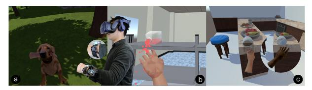
Fig. 1. Douleur is a wearable prototype that induces pain sensation of different intensity to enhance the immersion of realistic VR experiences: (a) The dog-biting scenario; (b) The corrosive liquid scenario; and (c) The spilled hot coffee scenario.
