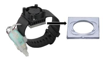
Fig. 5. Douleur prototype and the microfluidic channel.
