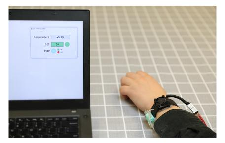
Fig. 7. The study setup: the experimental software controls the temperature change and pumps the capsaicin solution. When temperature reached a target level and was stable, participants were asked to rate their perceived pain intensity and type.
