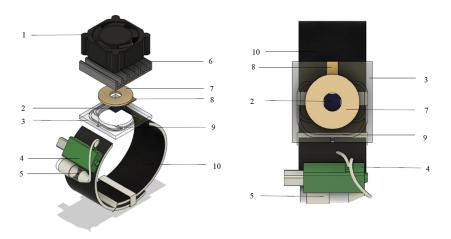
Fig. 4. Design of Douleur: 1 - Fan; 2 - Microneedling; 3 - Microfluidic Channel; 4 - Micropump; 5 - Reservoir; 6 - Heat Sink; 7 - Peltier; 8 - Temperature Sensor; 9 - Chemical Delivery Layer; 10 - Wristband.
