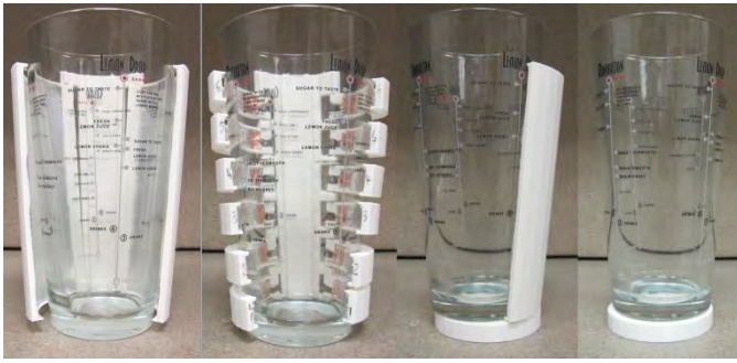
Fig. 2. Implementation of four capacitor designs and their placements on a glass cup.
