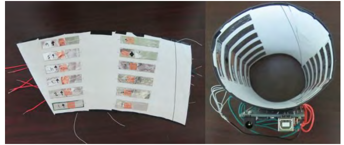
Fig. 4. A soft sleeve design with paper and electric tapes as the main support materials.
