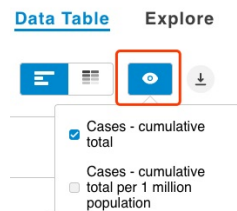
Figure 5.: The visual affordance of the “eye” icon, which was a button, mismatched with its actual function, which was a drop-down list.
