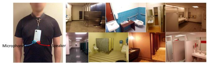
Figure 1. (Left) Wearable phone attachment for performing and analyzing impulse response and image capture; (Right) 8 sample restrooms used in our study.
