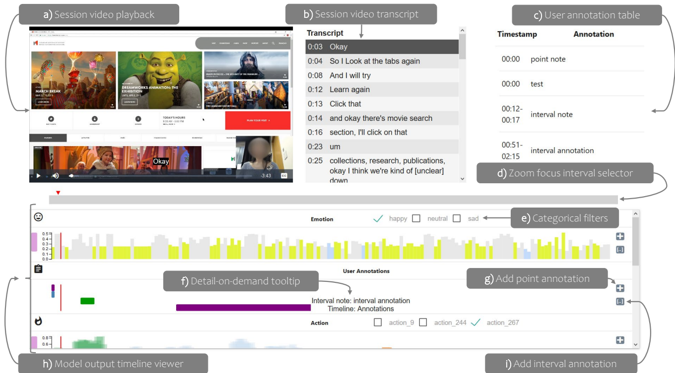
Fig. 1: Schematic overview. Analysis interface in the UXSENSE web-based client (view reflects tutorial video). a) Video playback: View user session video, with or without captions. b) Session transcript: View timestamped transcript of speech from video, and navigate video by clicking on line of text. c) User annotation Table: View the text and timestamp of all annotations made by the user. d) Zoom focus: Select, zoom, and pan whole extent of the video. Red arrow marker indicates current video time, while brushed region shows zoom extent in context of video duration. e) Categorical filters: When selected, non-selected elements of the view are shown with low opacity. f) Details-on-demand: Mouseover to get details of observation in model output at given time. g) Point annotation and i) Interval annotation: Add an annotation corresponding to given timeline for either the video’s current time ( g ) or the brushed interval range ( i ) with ( d ). h) Model output timeline viewer: The timeline and user annotations are described in Section 3.4.
