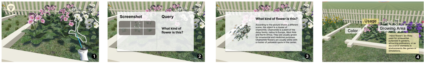
Figure 1: Probe 1: (1) Select the object and use audio to input the query; (2) System automatically screenshots six view pictures and sends them to Vision LLM along with the query; (3) Display 1: Vision LLM’s text results show along with the 3d object; (4) Display 2: Label Display.
