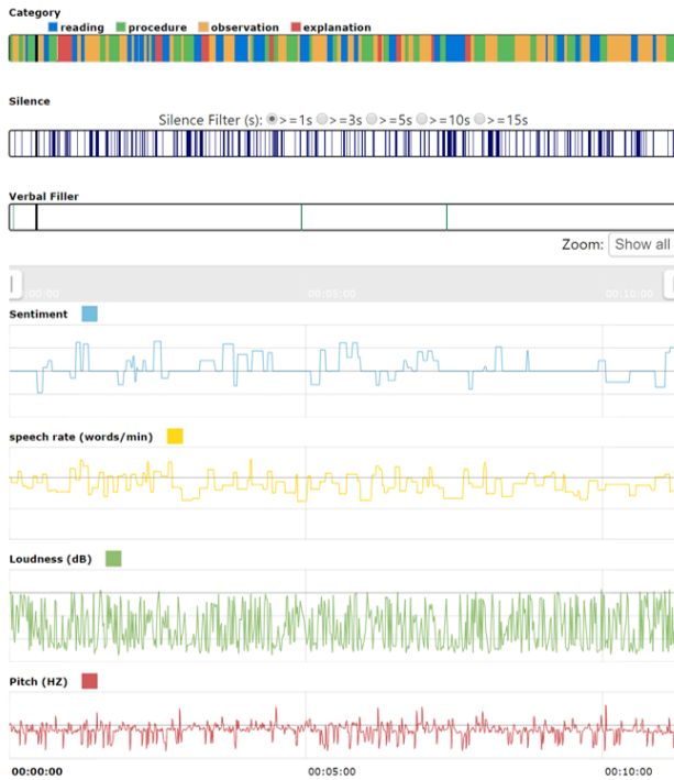
Fig. 2: An early version of VisTA that visualizes the verbalization and speech features of the entire think-aloud session to UX evaluators.
