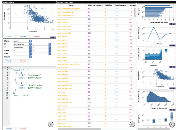
Fig. 9. The Baseline user interface consisted of a: (a) Chart Inspection Panel, (b) Data Table View, and (c) Chart List View, with similar functionalities to ChartSeer’s related panels.
